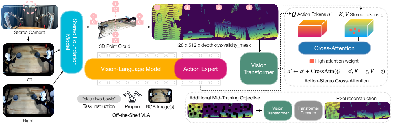
Fig. 2: Overview of ExStereo. ExStereo enhances pre-trained VLA models by leveraging a stereo camera and a pre-trained, frozen stereo foundation model [12]. Given a stereo image pair, the stereo model predicts a disparity map, which is converted into a metric depth map and 3D point cloud using the camera intrinsics and stereo baseline. We render the point cloud from four orthogonal viewpoints (Top, Front, Left, and Right) using z-buffering. Each view is rasterized at a resolution of 128 \times 128 and contains depth, 3D coordinates, and a validity mask. The four views are horizontally tiled into a multi-view observation of size 128 \times 512 \times 5 , then processed by a Vision Transformer (ViT) [5] to extract stereo tokens z . We leverage z for action generation through our proposed action-stereo cross-attention, where action tokens a' query z to selectively retrieve relevant 3D visual features while leaving the VLA’s prefix sequence and VLM weights unchanged. To learn robust 3D representations, we introduce mid-training with masked autoencoding (MAE), where the VLA reconstructs randomly masked multi-view patches from a large-scale stereo dataset while learning action-relevant features from incomplete observations. During VLA post-training, the ViT and action-stereo cross-attention block are frozen to prevent overfitting to task-specific demonstrations, while the MAE decoder is discarded.
